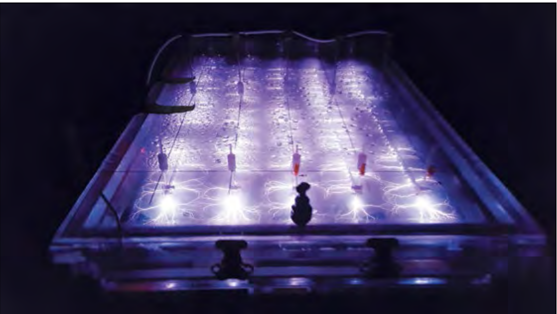
A plasma reactor is demonstrated Sept. 25 at Wright-Patterson Air Force Base, Ohio, to degrade and destroy perfluorooctane sulfonate and perfluorooctanoic acid, better known as PFOS and PFOA, in sample groundwater.
